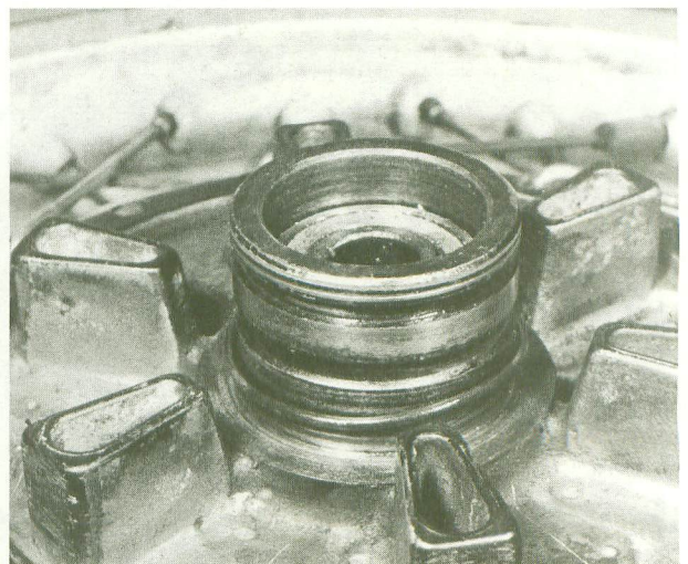
19.4a Do not omit the inner O ring on reassembly
