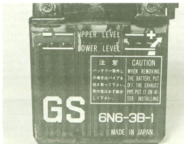
6.2 Electrolyte level is easily seen through transparent casing
