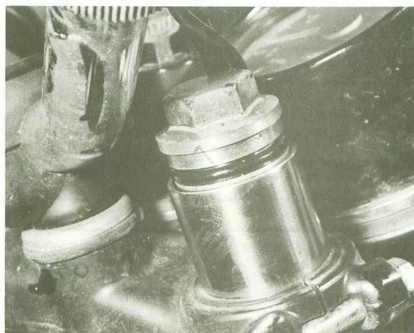
7.2b Do not omit the O ring on the stanchion bolt
