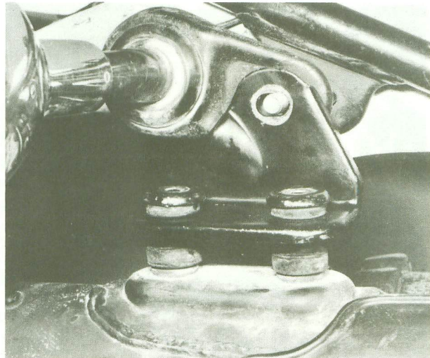
5.5c ... spark arrester support nut
