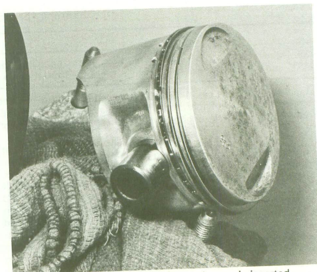
41.2a ... the piston is fitted and the gudgeon pin inserted
