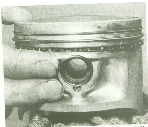
41.2b Install new circlips, ensuring their correct engagement
