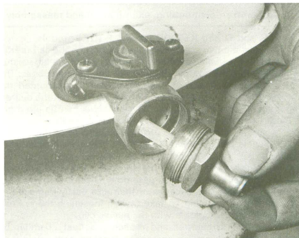
3.2b Secondary filter is used on some types of tap
