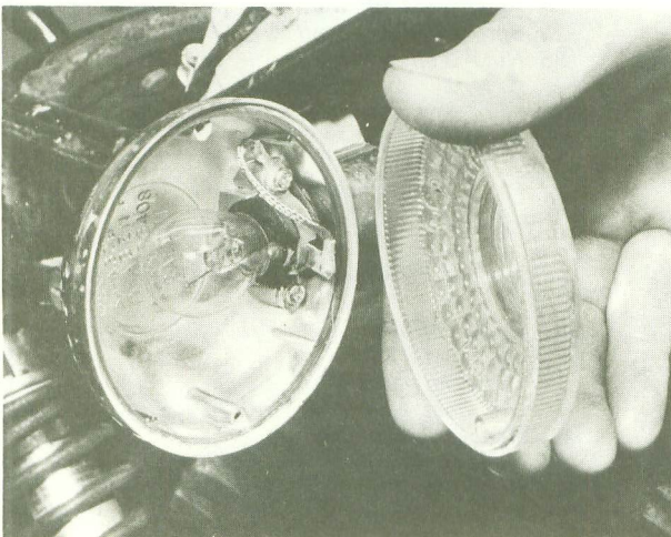
11.2 Flasher lens is held by two screws
