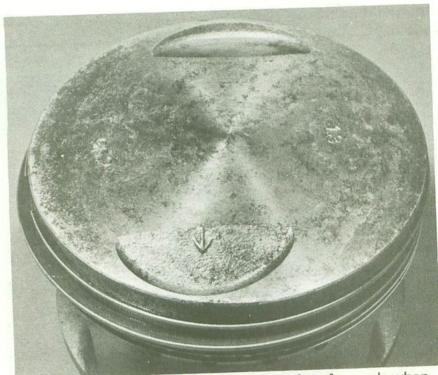
41.1 The arrow on the piston crown must face forwards when ...
