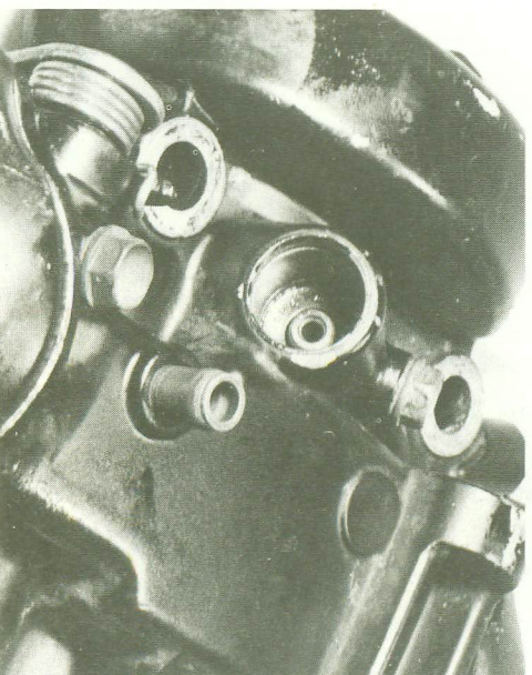
26.2 Tachometer drive shaft is secured in tunnel by a bolt
