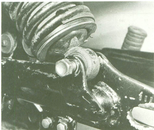
11.6 Detach the lower end of each suspension unit
