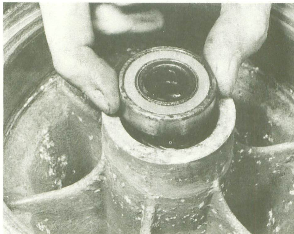
12.2 ... access to the wheel bearings; note seal side is outwards
