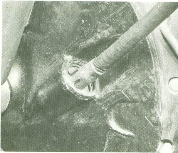
4.2a Prise out the circlip and ...
