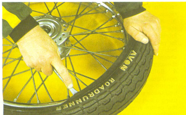
Use similar technique for second bead, finish at tyre valve position
