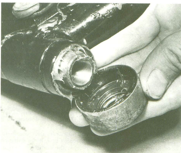
11.8b ... pull off the bearing cover from each side
