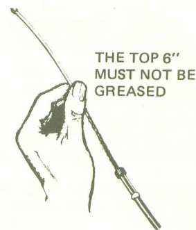
Greasing the speedometer cable
